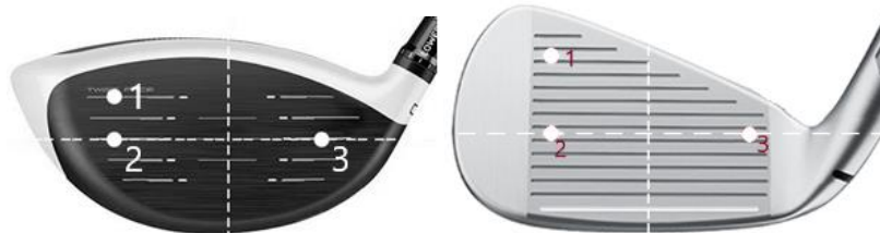
Figure19 Attachment of wooden and iron marking points
